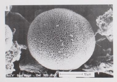
Phot. 8. Sulphate sphaerulite with honeycomb crystal fabric. Crystals are empty inside. SEM micrograph
