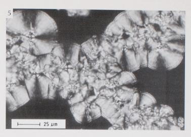
Phot. 5. Calcite sphaerulites and hemisphaerulites. Note smooth external surfaces of sphaerulites and well developed uniaxial pseudocross. Crossed polars
