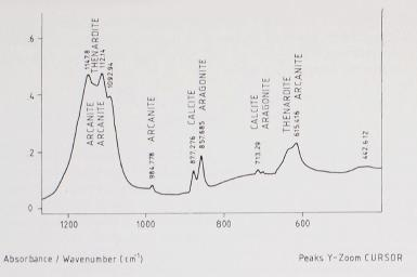
Fig. 3. Infrared absorption spectrum of some minerals from sample I
