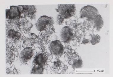
Phot. 7. Calcite raft with aragonite sphaerulites. Note spicular external surfaces of sphaerulites. Plane light
