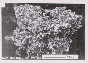
Phot. 1. Concretion of nesquehonite with perfectly developed crystals. SEM micrograph
