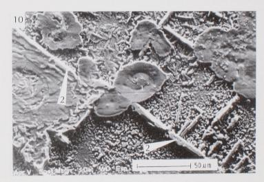
Phot. 10. Efflorescences of thenardite (1), and skeletal crystals of halite (2), analysed with EDS. SEM micrograph
