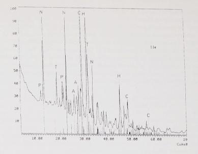
Fig. 4. X-ray diffraction pattern of minerals from sample II N — nesquehonite; H — halite; P — picromerite; T — thenardite; A — aragonite; C — calcite
