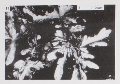
Phot. 11. Efflorescences of sulphates, wavy extinction well visible. Crossed polars
