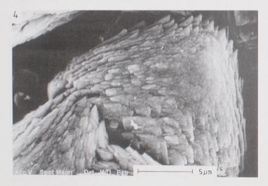
Phot. 4. Calcite rhombohedron built up of thin plates that are not parallel to each other. SEM micrograph
