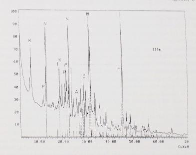
Fig. 5. X-ray diffraction pattern of minerals from sample III H — halite; N — nesquehonite; K — konyaite; P — picromerite; T — thenardite; A — aragonite; C — calcite
