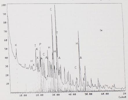
Fig. 2. X-ray diffraction pattern of minerals from sample I. H — halite; C — calcite; A — aragonite; T — thenardite; P — picromerite; X — hexahydrite; K — konyaite
