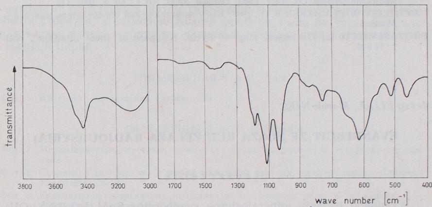
Fig. 1. Infrared absorption spectrum of svanbergite
