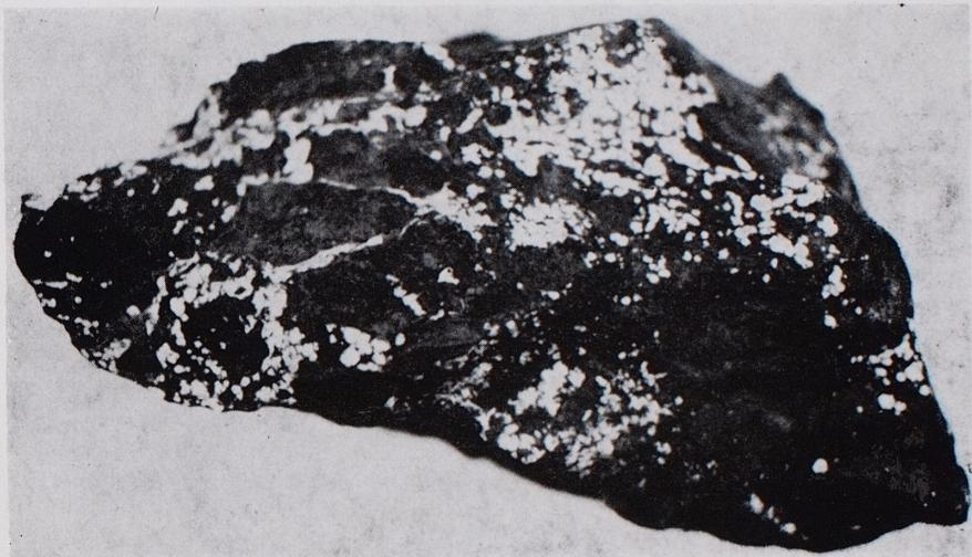
Phot. 1. Fine-grained svanbergite aggregate in limonitic ore. Natural size
