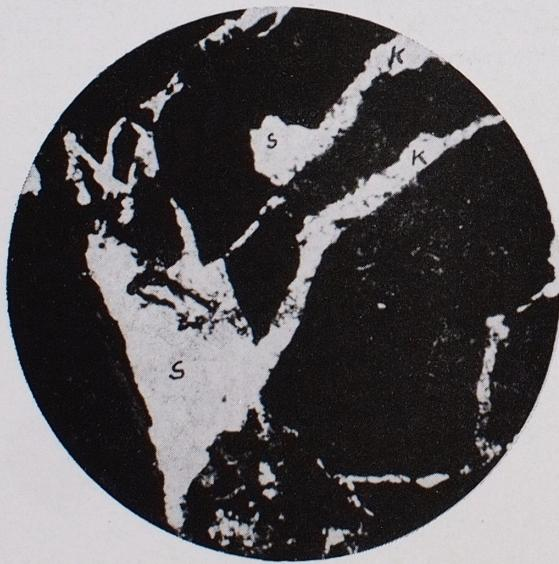
Phot. 3. Calcite-svanbergite stringer lodes in limonite ore. K — calcite, S — svanbergite. Magn.  $\times 30$
