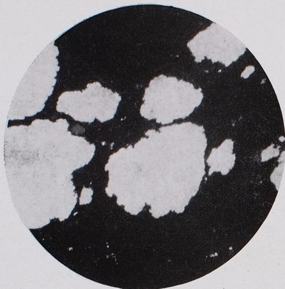
Phot. 2. Concretional svanbergite aggregate. Partially crossed nicols. Magn.  $\times 30$
