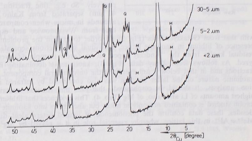
Fig. 3. X-ray patterns of size fractions separated from residual kaolin from "Antonii" open pit in Zarów (sample 3Z)
